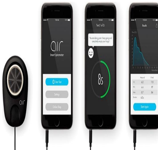
Figuer:3. Air smart spirometer after 6 seconds of exhalation, the chronometer turns green
